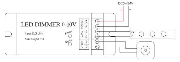
2. External connect 0-10V voltage dimming
